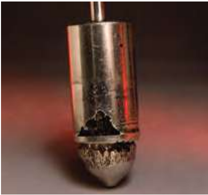
Figure 5.8 Typical Appearance of Flashing Damage
