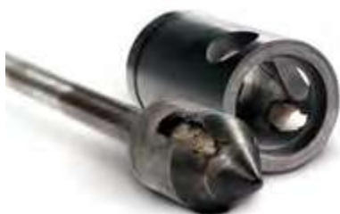
Figure 5.9 Typical Appearance of Cavitation Damage
