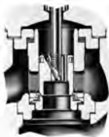
Figure 3.36 Adapter Method for Providing Reduced Flow Capacity
